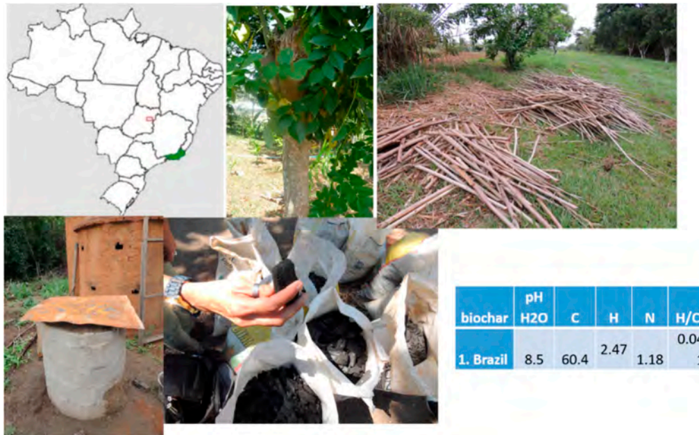
Figure 1. Steps of production: Rio de Janeiro state where biochar was produced, Gliricidia tree, dry Gliricidia before being cut at put into the stove, drum stove, biochar (before being sieved), table with biochar properties [4].
